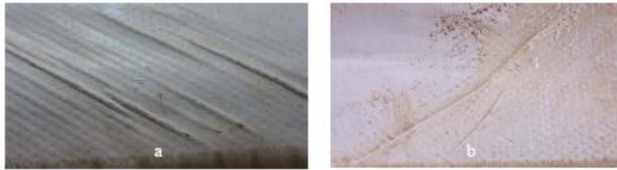
Figure 3: membrane damage (folds) near the (a) feed and (b) concentrate sides of membrane envelope.
